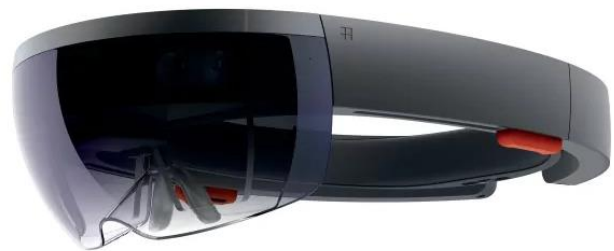
Figure 2: Image of the HoloLens (Microsoft, Redmond, WA, USA) as used in the presented mixed reality application (Source: microsoft.com)
