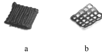
Figure 2: 3D nanocomposite bioconstructions obtained from a grid trajectory with a distance of 0.5 mm (a) and 1.5 mm (b) between parallel lines
