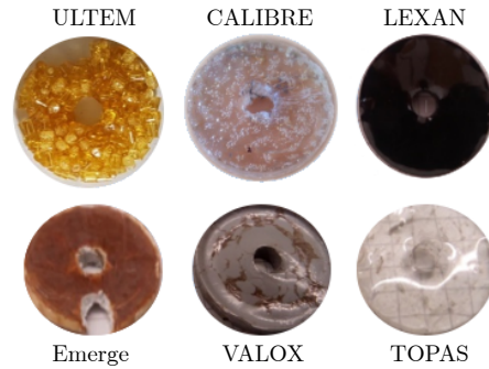
Figure 2: Materials after initial mold test in which the granulate was heated to its transition temperature
