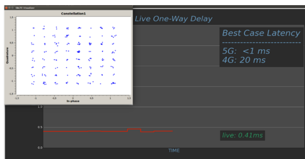
Figure 2. Latency of 5G data transmission can be reduced to < 1ms by carefully selecting the transmission parameters. The measured signal delay of the deployed 5G module including encoding and decoding was 0.41ms.
