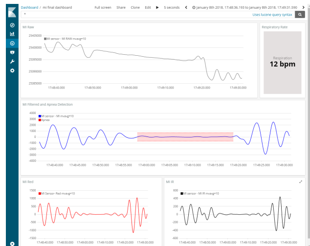
Figure 6: Visualisation of magnetic induction (MI) signal based on Kibana visualisation plugin for Elasticsearch and AngularJS platform [6].
