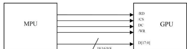
Figure 3: 8080-series Bus Interface
