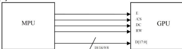
Figure 5: 6800-series Bus Interface
