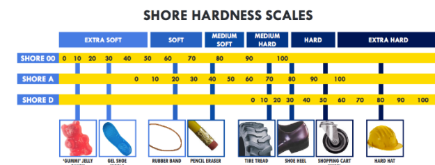
Figure 2: Shore hardness scale
